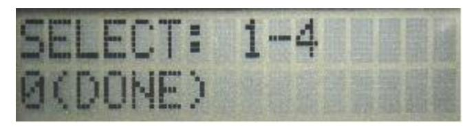
This step is where you must program your input channels for Normally Open (N.O) or Normally Closed (N.C) contact activation.
