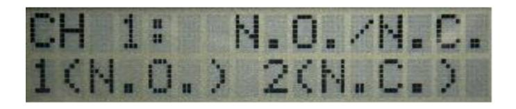
N.O. is Normally Open and N.C. is Normally Closed **EC4** products are set N.C. Normally Closed If you purchased the **EC4**, Press 2 (N.C.).
