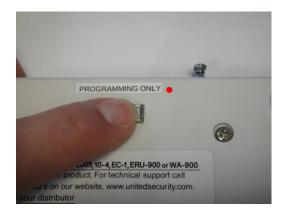
6. Once you see the LED blinking on your PS1 transmitter, hold down the red button on your PS1 transmitter for about 1-2 seconds to activate your P1S transmitter.
