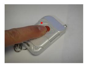
7. The LED will stop blinking and your P1S transmitter has been paired with the EC4 Dialer.
